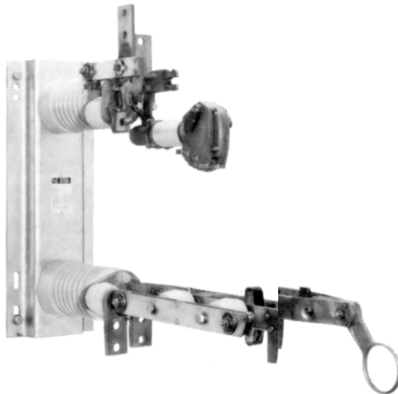
Figure 4 - Switch fully open. Voltage-regulator magnetizing-current interruption has taken place within the interrupter with no external arc or flame. Voltage regulator is de-energized and bypassed.
