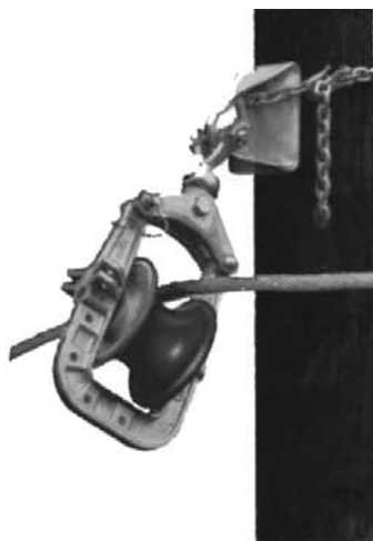
Aerial Cable Block
