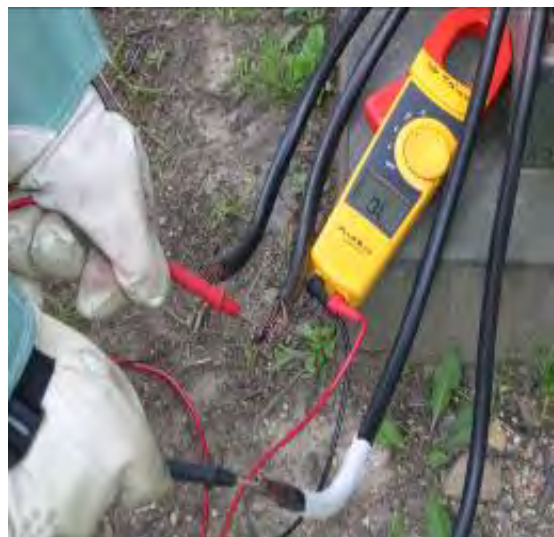
Opposite Conductors Open Link OL No Continuity
