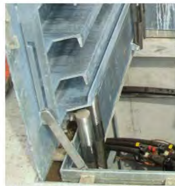
View of locked open hatch, to close latch, push locking arm inward then apply pressure onto hatch to close it
